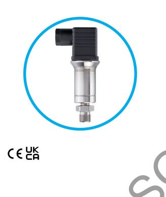
The external mount hydrostatic level transmitter, ILSE, has a piezoresistive silicon pressure sensor which is an oil filled isolated diaphragm. The sensor and housing are made from stainless steel with a choice of internal 0 ring seals to ensure the product is suitable for a wide range of applications.
