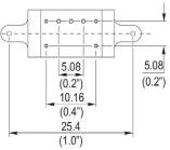
The following Pins require 0.9mm diameter  $\pm$  0.05mm holes, where fitted 1, 2, 5, 6, 7, 8, 9
