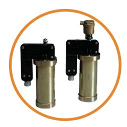
The switch is based on a simple principle of a float located inside an enclosed chamber, which follows the level of the liquid in the system. When the liquid level rises, the float magnet attracts and operates a 20A 250Vac microswitch with N/O and N/C contacts. Suitable for use in water or liquids of SG equal to or greater than 1.
