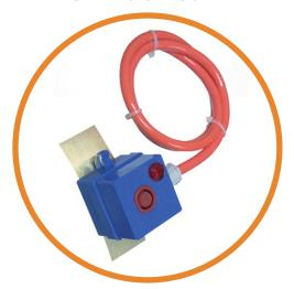
The FCTE is a heat sensor, which is attached to the outlet pipe from a pump. This device works by reacting to the temperature at the outlet of any centrifugal type pump, which will rapidly rise past 45° if the inlet water level falls below the centre line of the inlet. The unit will cut off the electrical supply to the pump, so protecting it from damage. Manual resetting of this unit allows the pump to restart.
