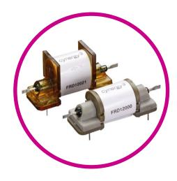
An open frame RF reed relay with 8kV isolation and 6A (at 30MHz) carry current, the FRD12000 series has been used in many HF radio systems over the years, with applications in commercial maritime (GMDSS) equipment and military HF radio units worldwide. The use of vacuum reed switches with rhodium contacts offers high isolation voltages, low contact resistance and long operating lifetime.
