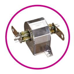
The very high carry current capacity and high voltage isolation of this series is achieved through the use of multiple high vacuum reed switch contacts, ensuring a high level of performance and reliability. The two standard models will carry currents of 12 and 20Amps respectively at 30MHz and feature silver plated, fully screened coil assemblies for ultralow RF losses. Typical applications include over the horizon (OTH) HF radar systems and 1kW base station transmitters.
