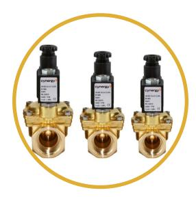
The SOL Series is a range of 2-way solenoid valves which are pilot operated and are available in a choice of 110Vac, 230Vac or 24Vdc coils to suit the required voltage.
